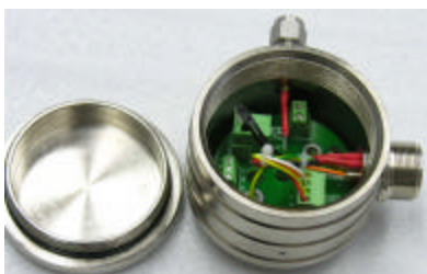
5. Termination Head & circuit board
